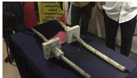
Figure 2. Thread-bar on the pier-head formwork bracket for the Becakayu Toll Road Project
