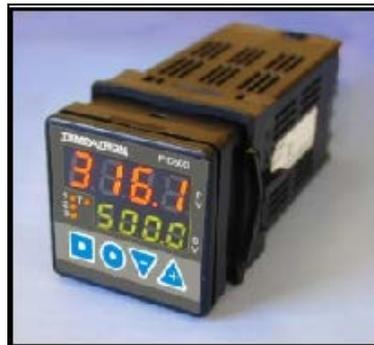
**Gambar 2.6** PID Controller
