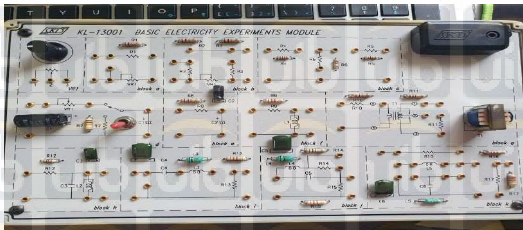
Gambar 4.11. Module KL-13001 Basic Electricity Experiments Module
