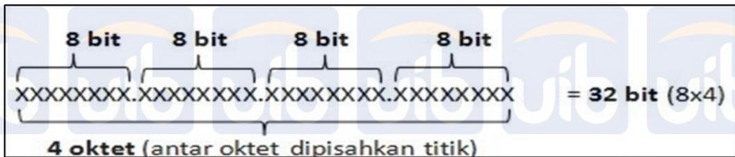
Gambar 2. 7 Format penulisan IP Address
