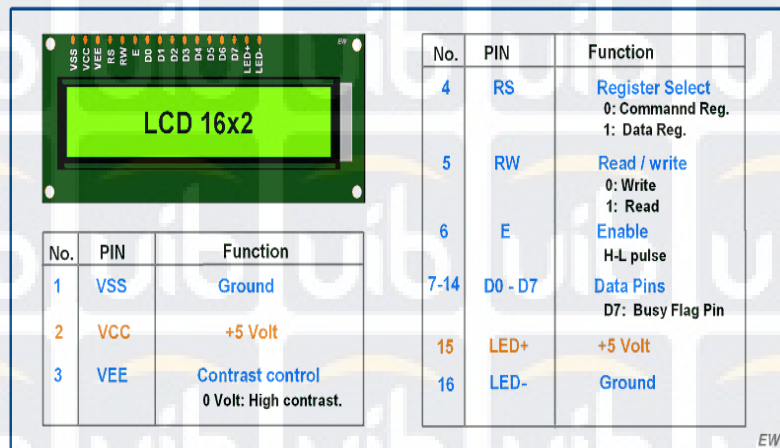
Gambar 2 . 25 Definisi pin LCD 16 x 2
